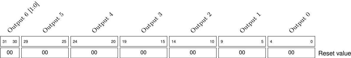
Figure 3.36: SafeSU - Crossbar Configuration Register 0 (0x0AC)
